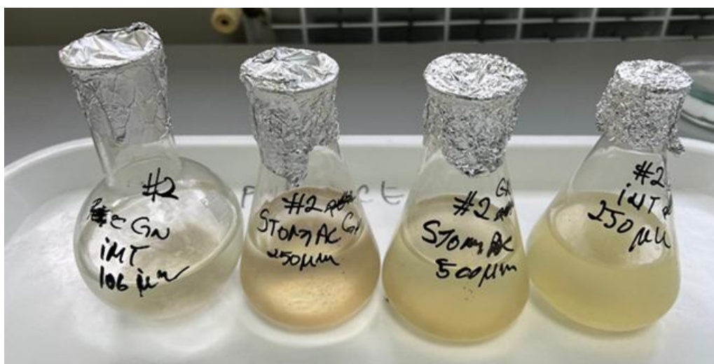
Figure 30 Samples of GIT contents after incubation with KOH solution
