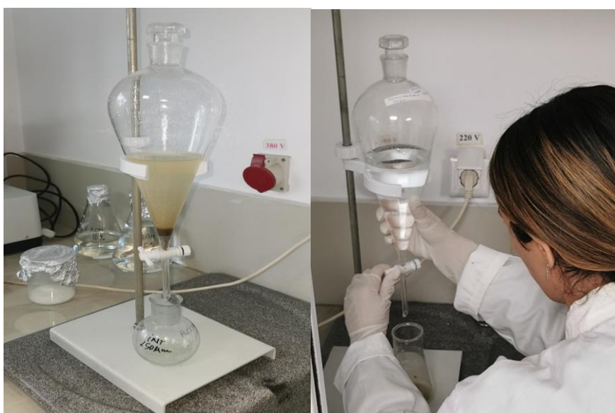
Figure 32 Separation step with NaCl saline solution
