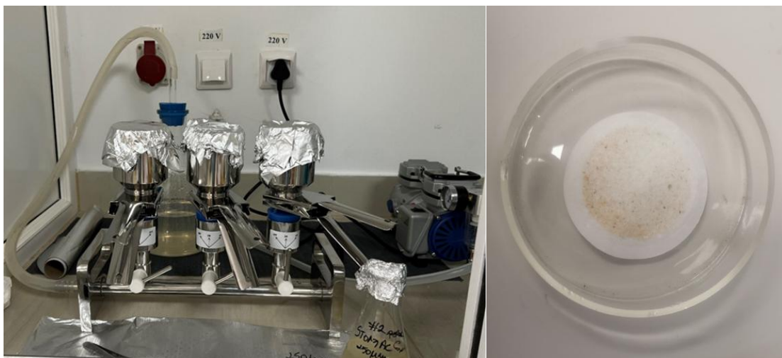
Figure 31 The stage of filtering the samples and drying the filters in Petri dishes
