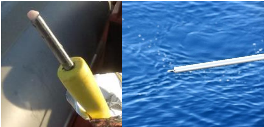
Figure 6. Arrow and tip (left) and tip on the aluminum pole (right) with the collected biopsy.
