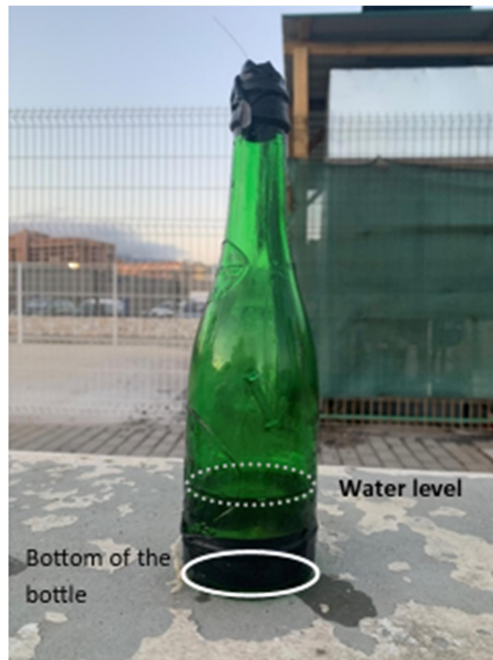
Figure 13. Glass bottle partially filled with sea water. Water filtered through the cork due to the water pressure.
