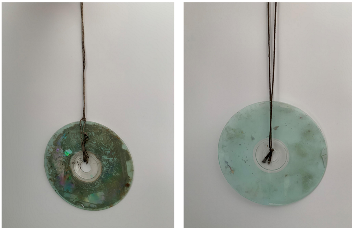
Figure 19. Images of the wear and tear of the CDs after their installation in the nets.
