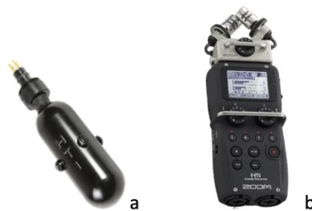
Figure 8. Instrumentations used for the acoustic data collection: a) HTI-96-MIN marine-mammal hydrophones; b) Zoom H5 handy recorder.
